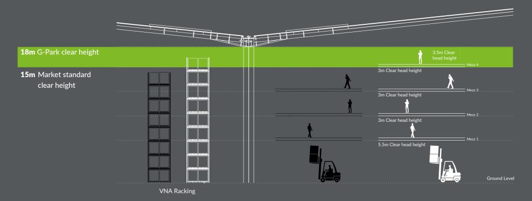
Increased racking height with VNA Increased mezzanine floor capacity
