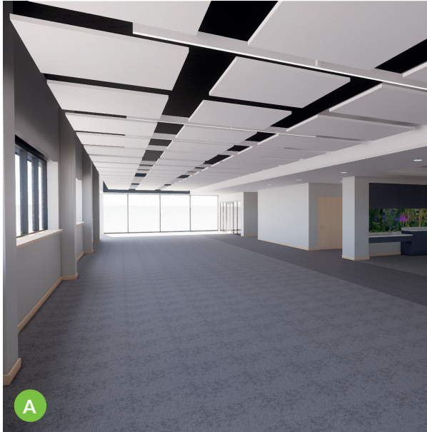
Exposed ceiling with acoustic panels and strip LED
